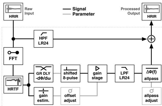
**Figure 5:** Basic structure of the adaptive LFE algorithm. frequency extension (LFE) algorithm has been employed that generates the low frequency component and matches gain and phase, see Figure 5. Each HRIR and each ear is processed independently. At certain crossover frequency (200 Hz) the original HRIR is high-passed
