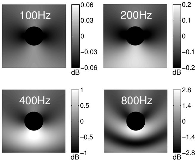
**Figure 4:** Analytic simulation of the pressure magnitude at different frequencies for a plane wave impact with unit gain from south to a rigid sphere with a typical diameter of 17.5 cm serving as a simplified model of the dummy head. Below the LFE crossover frequency of 200 Hz, the magnitude deviations on the sphere surface are already less than  $\pm 0.2$  dB.
