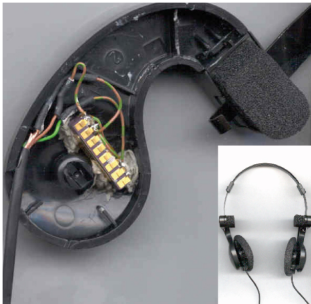
Figure 3: The sensor was integrated into a Koss headphone and (later) clad with casting resin.
