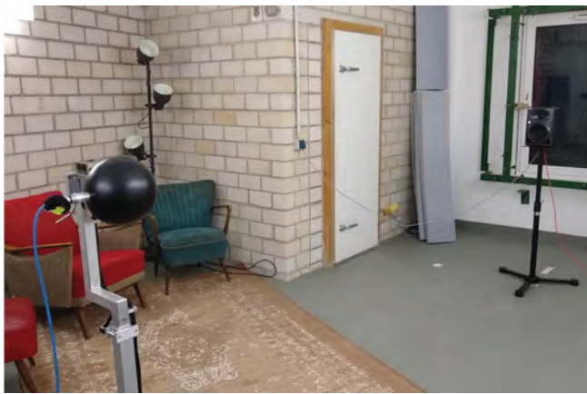
Figure 2: Photograph of the Audiolab showing the measurement setup of source position LSC and receiver position 1. It shows the VariSphear with rigid-body extension and the Neumann KH120 loudspeaker.
