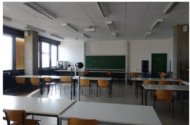
Figure 4: Photograph of the Classroom showing the VariSphear at position 1 and the Neumann KH420 loudspeaker at position LSR.
