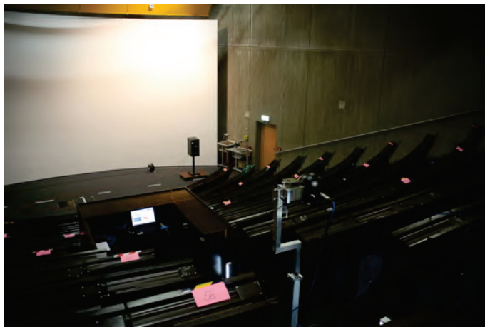
Figure 6: Photograph of the Audimax showing the VariSphear at position 1 and the Neumann KH420 loudspeaker at position LSR. The sound source is slightly elevated downwards.
