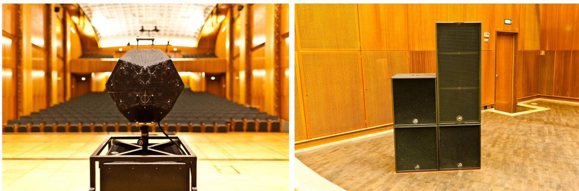
**Figure 18** Omnidirectional source: The high power wideband dodecahedron "Sonic Ball" (left picture) and the horn loaded PA rig from AD-Systems (right picture)
