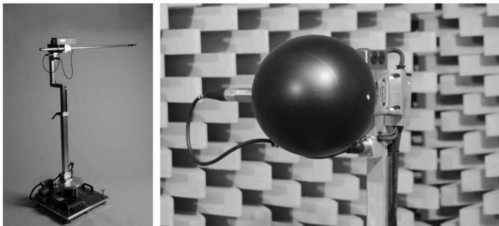
**Figure 12** *VariSphear* scanning array system in an open sphere configuration (left picture) and with the rigid sphere extension and the Earthworks M30 microphone (right picture).
