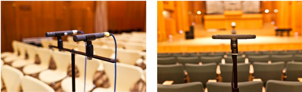
**Figure 14** Example for a stereophonic configuration (left picture: Small AB with Schoeps MK2, right picture: ORTF with Schoeps MK4)
