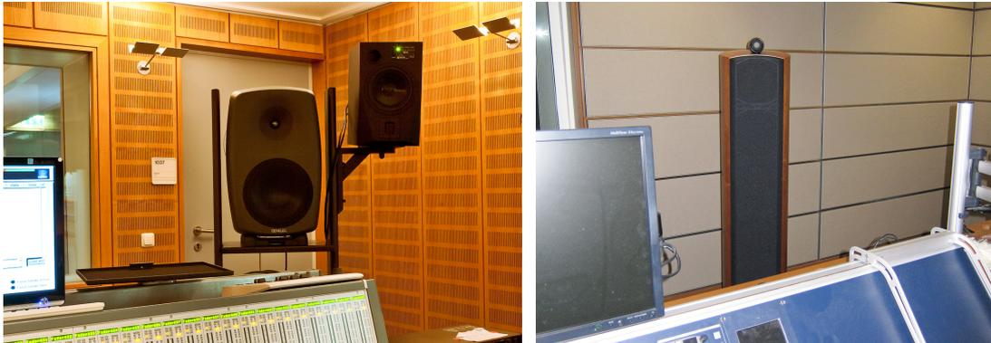
**Figure 17** The used main monitor systems: Genelec 8260A in CR1 (left picture) and B&W 803D in CR7 (right picture)
