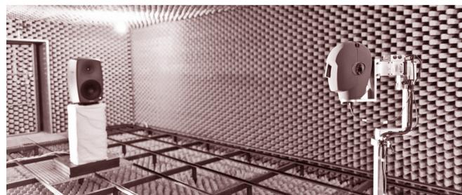
**Figure 1:** Genelec 8260A speaker and Neumann KU100 dummy head mounted on the VariSphear motion system [5] in the anechoic chamber. [Photo: P. Stade]
